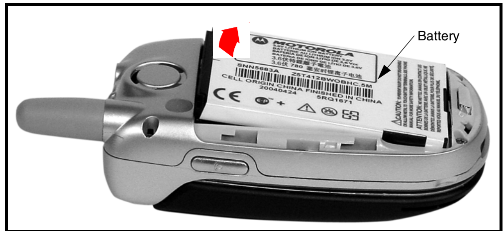
Figure 5. Removing and Replacing the Battery
